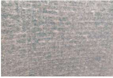
Manually laminated hand lay-up polyester resin fiberglass to controlled thickness.
